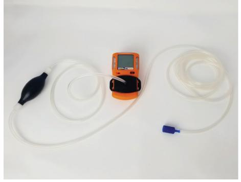
The probe is used for probing in confined spaces, crawl spaces, equipment rooms, etc.
