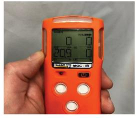
The detector will then scroll through a series of info; last calibration, last bump, and the readings in the detector.
